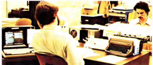
The latest newsroom facility consists of eight terminals similar to the one seen here (in the foreground) and a distributed processor in the corner of the room. This is one of two stations in the newsroom, each having three terminals. The assistant editor (back to camera) tapes an interview preparing for a new update. Editor Jim Cullen (right) checks a new story on one of the other terminals.
